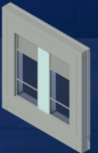
Non-structural Façade Panel
