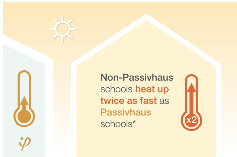
\*Internal air temperature increased 1.6°C (per 4°C external warming), compared to 0.8°C in Architype's Passivhaus schools.
